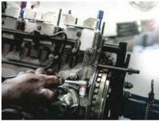
Nutsetter for hexagon head screws
